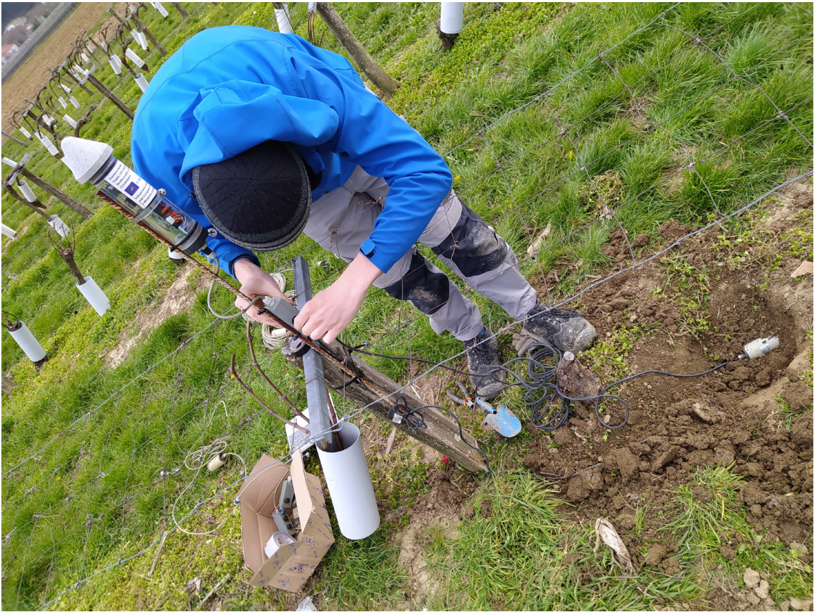
Picture 5 Installation of water level meters in terrain within the project LIFE Vi-VaCCAdapt LIFE15 CCA/SI/000070 (Author: Luka Žvokelj)
